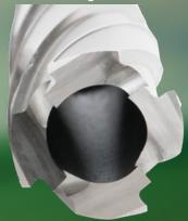
Re-sharpened cutter restored to factory geometry
