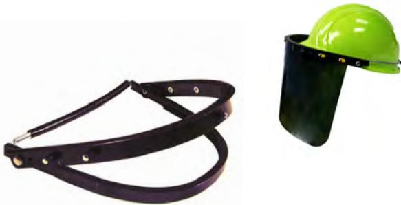
Aluminum mounting bracket with universal locking cams for easy window installation and removal. Position-stop friction joint that holds the visor in the desired position. Bracket fits most conventional hard hats.
